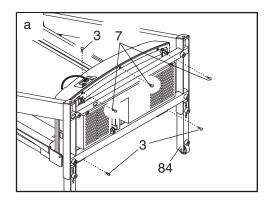
With the help of a second person, carefully raise the Uprights (84) to the position shown. Carefully pivot the Hood (41) off.
